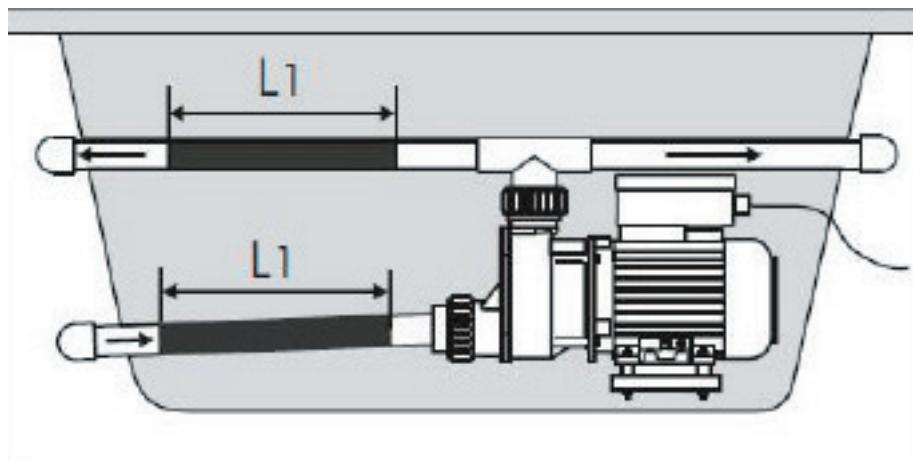
3. PVC pipe: (Fig. 3) cut a suitable piece of PVC pipe/hose from the pump's intake/outlet and mount it on the heater's fitting valve.
