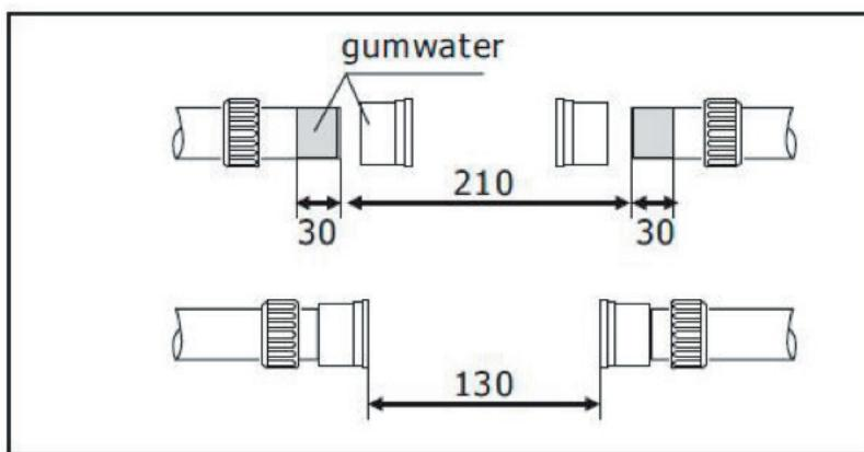
5. Installing the heater: (Fig. 5) Fit the hose to the heater's hose coupling. Make sure that the connection is completely tight. Please also note that the components are made from a plastic material and therefore can be broken if the couplings are over tightened.
