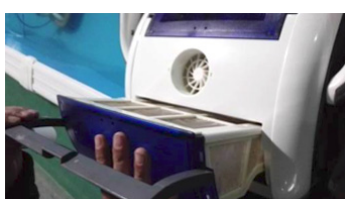
7. Slide the filter tray along the groove
