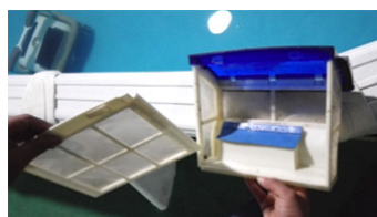
5. Pull out the filter panel vertically
