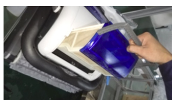
2. Lift the filter tray
